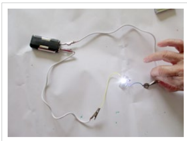
Figure 12. Completing an electric circuit
