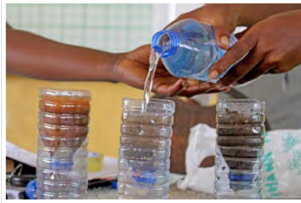
Figure 107. Testing water retention
